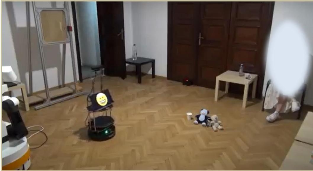
*Figure 19 - Turtlebot recognizing objects on the floor and interacting with a user.*
