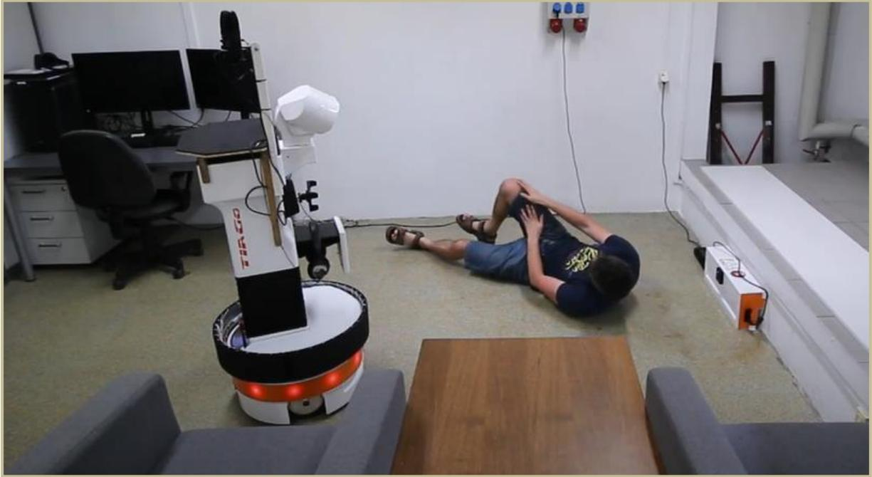
*Figure 16 - Tiago reacting to a human fall in a work office.*
