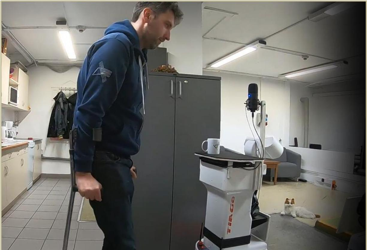
*Figure 17 - Tiago helping a person using crutches to transport a cup of tea.*
